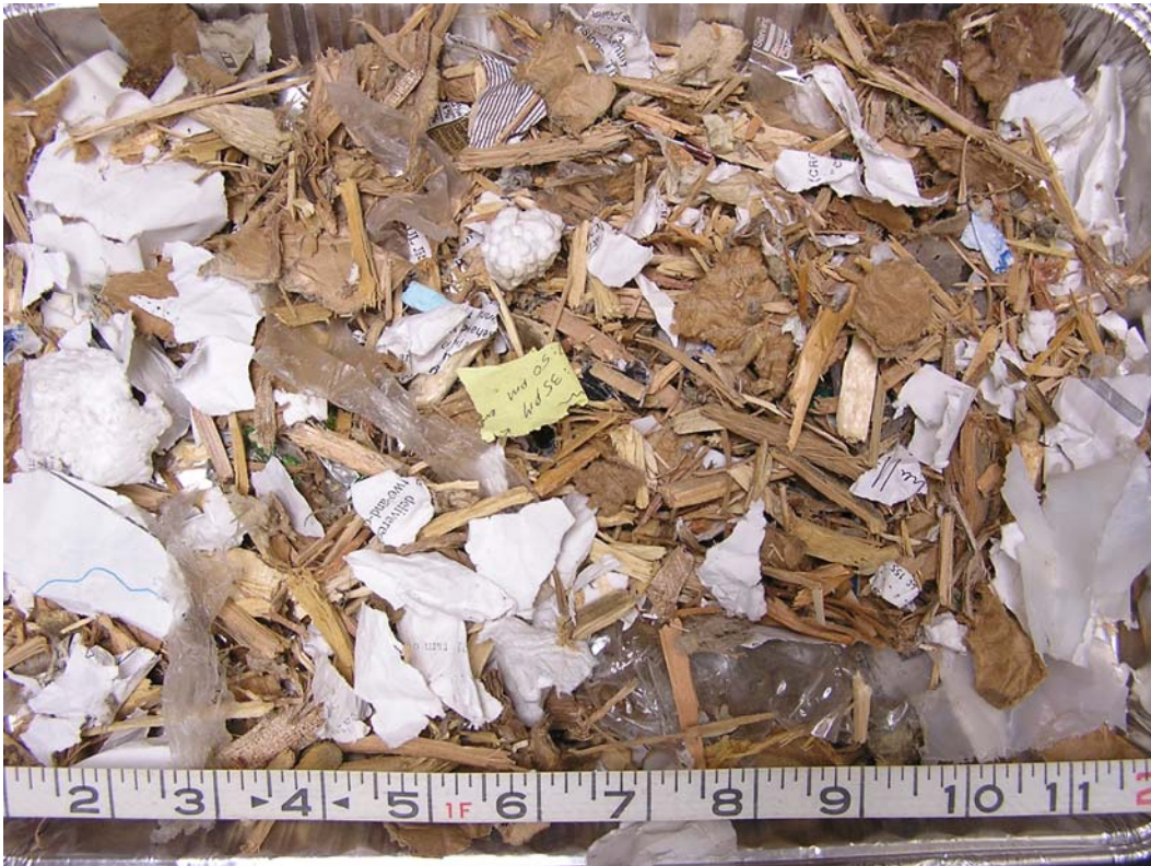
Figure 8. Unprocessed test material. This waste was shredded again in the lab to further reduce particle size prior to being placed into the reactor vessel.
