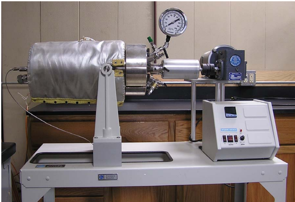
Figure 7. Parr reactor vessel used to mimic conditions inside hydrolyzer. Test material was kept at a set temperature within the heat-jacketed vessel on the left, while being constantly stirred by the motor on the right.
