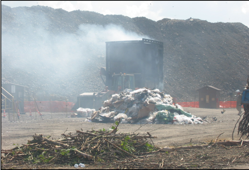
Figure 1. Smoking air curtain incinerator at a U.S. camp in the Balkans. The pile of material behind the incinerator is accumulated residue from the incinerator.
