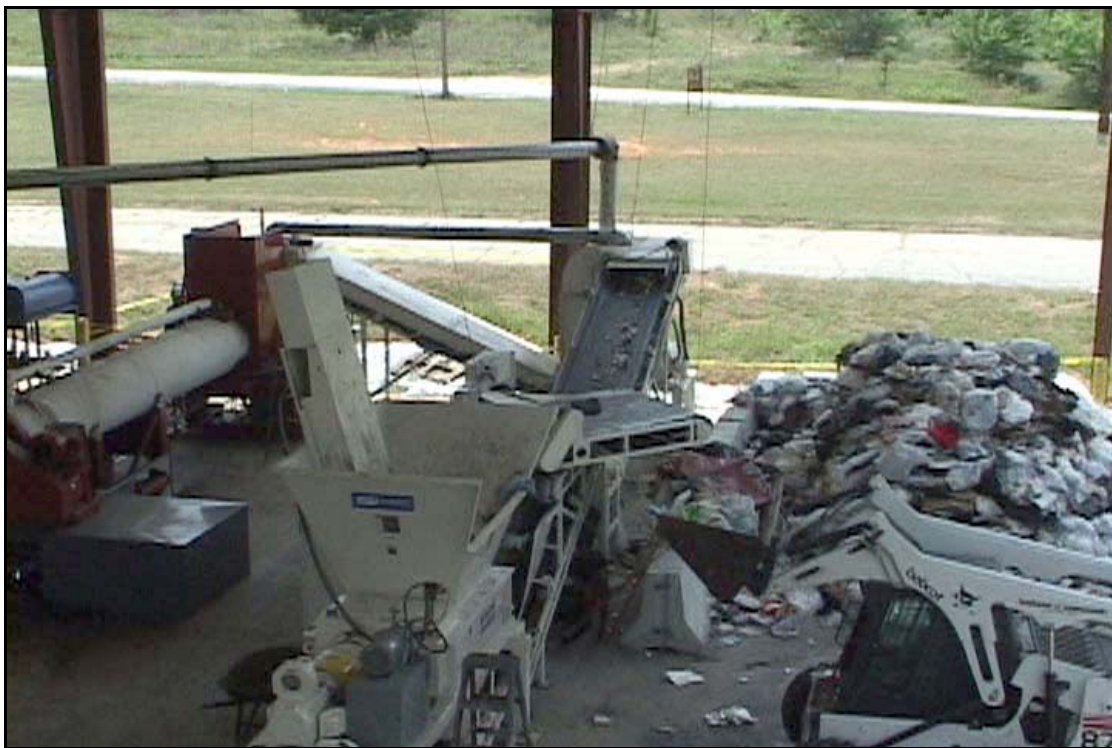
Figure 4. Bouldin processing system used during Fort Benning demonstration. A Bobcat is loading initial shredder with domestic waste from pile on right. Shredder is followed by metal removal, a second shredder, grinder, and hydrolyzer (on left).
